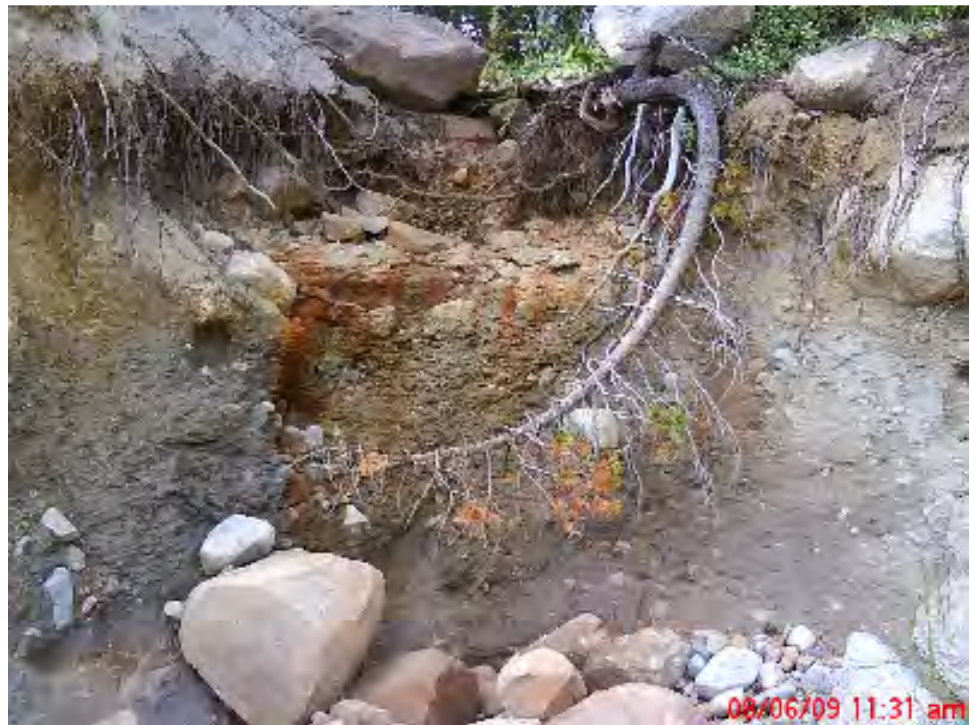
Figure 19 View of Glacial Moraine Deposits Located Next To Railroad Tracks (Consists of angular granitic rock clasts in a dense, silty, sandy matrix. Permeability is likely fairly low. This exposure is located on the drainage which originates on the east side of the runoff recovery pond. Note the near-surface iron stain.)
