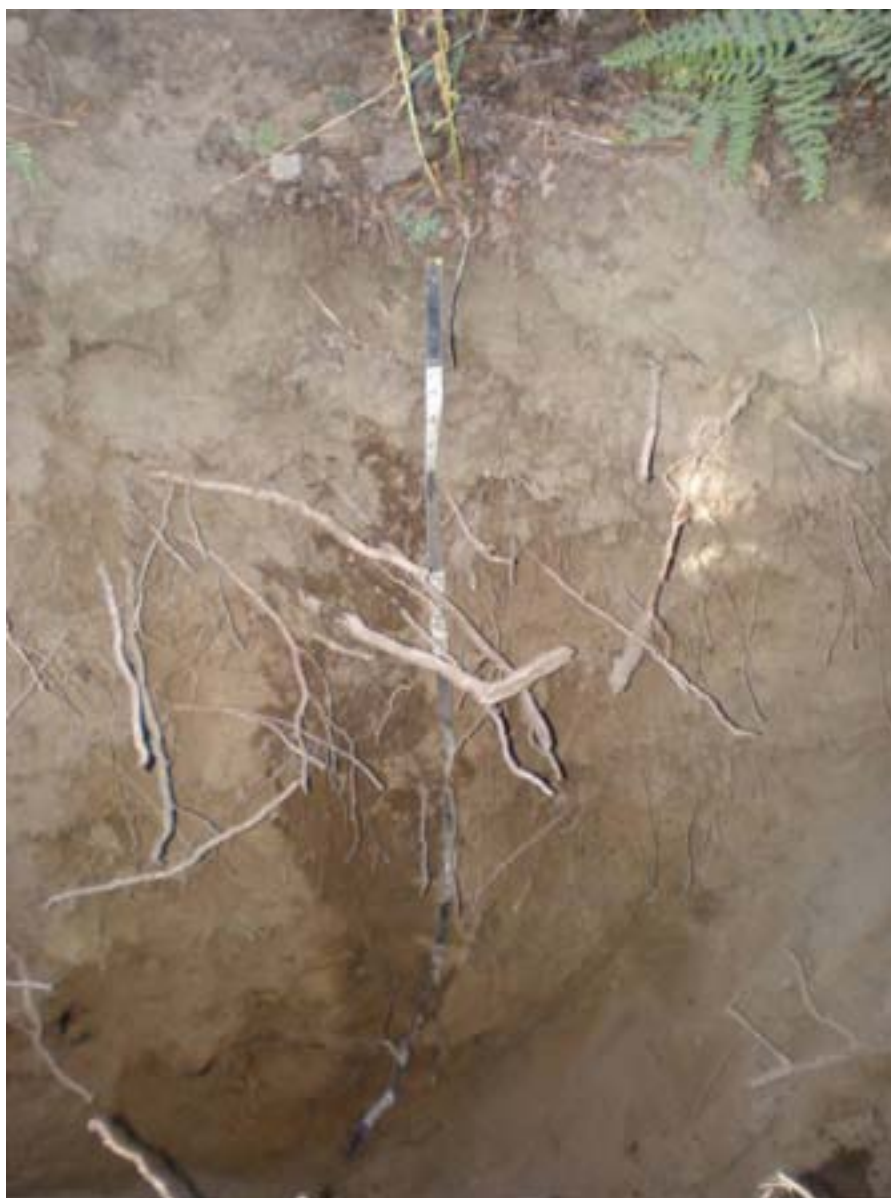
Figure 5 Profile of the Gefo Variant Exposed in Pit 3 (Divisions Represent 10 cm, Numbers are Inches)
